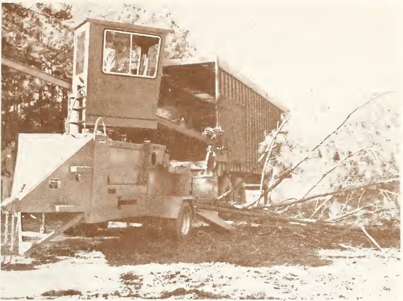
A mobile chipper converts whole trees into chips for better utilization.
